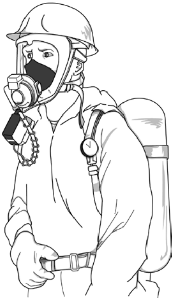
A self-contained breathing apparatus (SCBA) provides air from a cylinder carried by the wearer.
