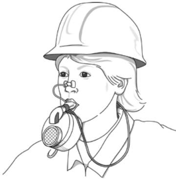
Bite blocks are often used by workers in ammonia refrigeration facilities, pulp mills, and chemical manufacturing plants.
